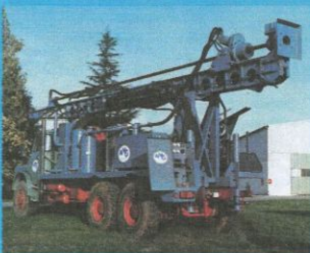
The TD 500 truck mounted drill.
