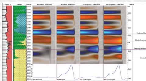
CSEM use a high-powered source to transmit low-frequency signals through the Earth to an array of receivers. By interpreting the received signals using forward modeling and inversion approaches, the resistivity structure of the seafloor can be determined. Resistivity well logs often show that commercial hydrocarbon deposits may be
