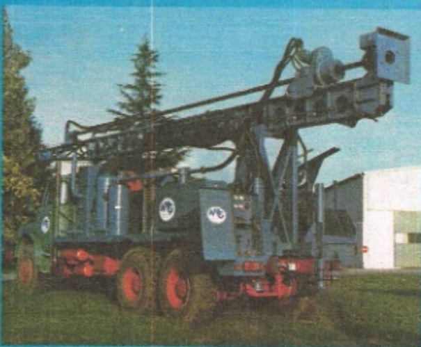
The TD 500 truck-mounted drill.
